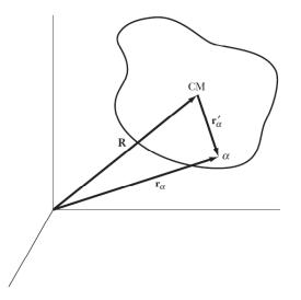
**Figure 7-1** – Description of the position of a particle using its position vector from the centre of mass of the system.
