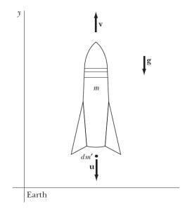
**Figure 7-3** – A rocket in vertical ascent under Earth's gravity. A mass dm' is ejected from the rocket engine, during a time interval dt, with a velocity **u** with respect to the rocket ship.
