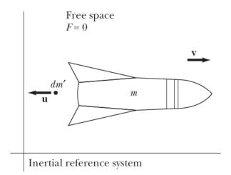
**Figure 7-2** – A rocket moves in free space at velocity  $\mathbf{v}$ . In the time interval dt, a mass dm' is ejected from the rocket engine with velocity  $\mathbf{u}$  with respect to the rocket ship.
