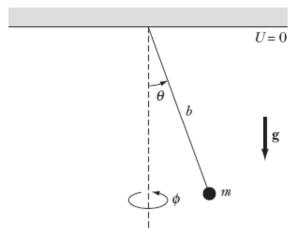
**Figure 5.1** – A spherical pendulum with generalized coordinates  $\theta$  and  $\phi$ .
